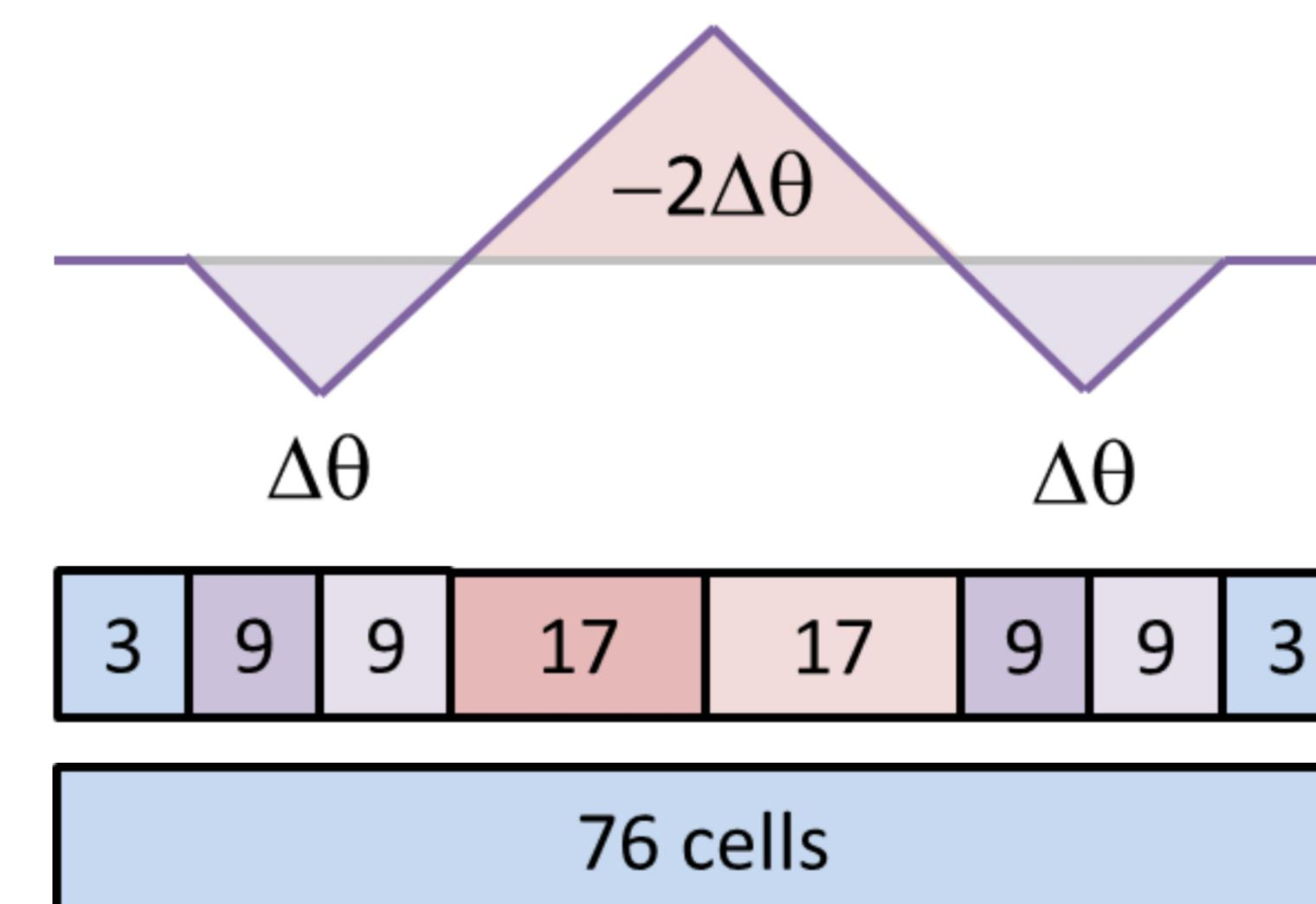
70 of the 76 cells of the eRHIC straight section may be divided up into ramps of increasing and decreasing curvature to give this variation in the required space. Tracking shows that the orbits return to the centre line as required, with a small error. This is shown below with a transverse exaggeration of 2000x.
