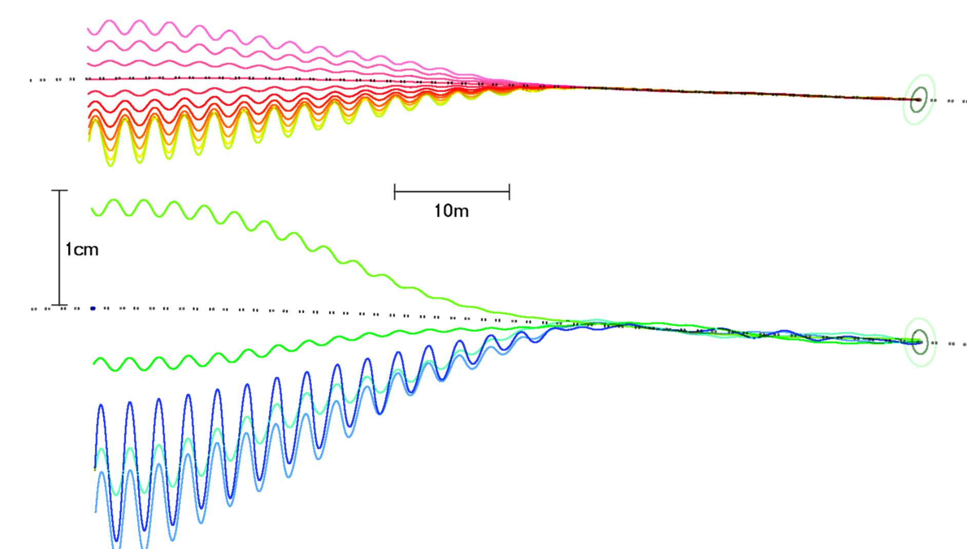
The orbits move smoothly towards the centre line as expected. As the transition is not infinitely long (and therefore only approximately adiabatic), there is some residual orbit oscillation left over in the straight sections, which amounts to  $\pm 0.436$ mm in the low-energy FFAG and  $\pm 0.066$ mm in the high-energy FFAG.
