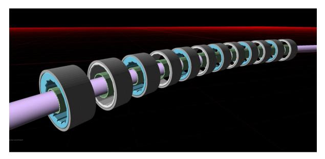
In order to fit the 4x energy range through the existing magnets, the lattice had to be carefully optimised to reduce the orbit excursion, allowing the beams to fit inside a simple toroidal vacuum pipe that fits in the magnets. The table below gives the critical radii and clearances in this construction.
