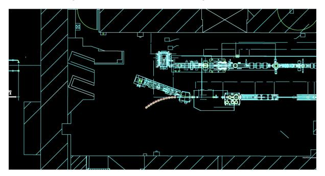
A zoomed in version (below) shows that the FFAG input orbits and angles are large compared to the ATF output pipe of this beam port. So it is probably necessary to make the table holding the FFAG able move sideways and rotate to put the output ATF beam down the nominal closed orbit for each energy. This requires a bellows on the vacuum connection and either manual or stepper motor movement. The 12 magnets only weigh 33kg in total so the mass of the table is not prohibitive.
