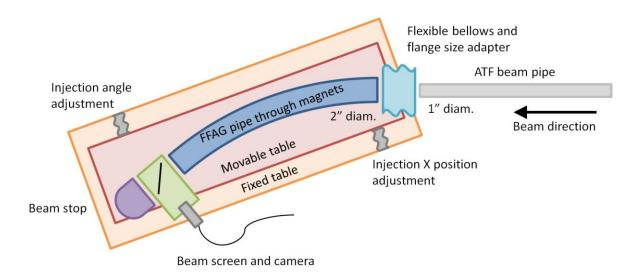
The ATF beam has some position/angle scanning capability but it comes from a smaller aperture pipe than the FFAG uses and thus cannot cover the full range of entrance positions and angles. The experiment provides additional adjustment of the injection position and angle by putting the entire beamline on a movable table (fortunately the beamline is very compact). This will only need to be adjusted per beam energy setting and can remain fixed for injection position/angle scans.
