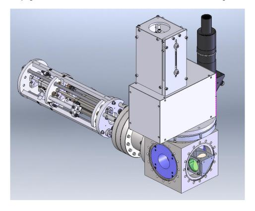
The cube (bottom right) is where the beamline flanges will be attached. It has a flange-to-flange distance of 6 inches. The arm for retracting the screen will not be operated for this experiment, as the screen is always the final element of the beamline, so being a destructive diagnostic is not a problem. While getting this diagnostic to work, it may be a good idea to temporarily attach it to the bellows at the beamline start (without the FFAG) so it can be tested on its own.
