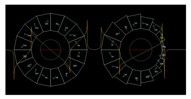
The magnets use the Neodymium-Iron-Boron grade N35SH from AllStar Magnetics and the current sheet simulation above uses an effective  $B_r$  of 1.194T (and  $\mu_r$ =1), which has proved a good fit to both OPERA-3D results and reality in terms of integrated field strength. The main parameters of these magnets are given in the table below.
