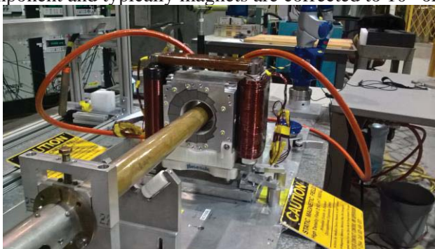
Figure 6. One of the tuned CBETA magnets being measured on BNL magnet division's rotating coil.
