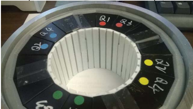
Figure 5. (left) Permanent magnet with tuning pack inserted. Variable length iron wires are visible in slots. (right) Summary statistics from field tuning of 216 magnets in the CBETA project.
