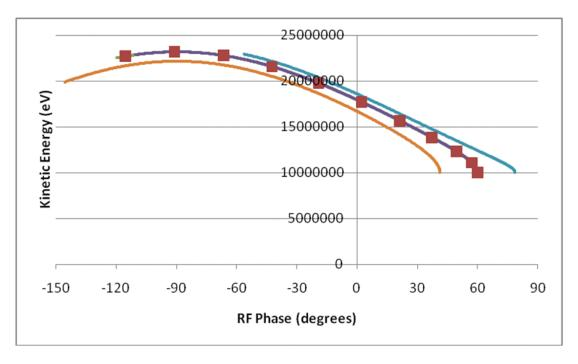
As the beam closed orbit has the same circumference at all energies in a scaling VFFAG, the time-of-flight for electrons in the ring simply scales as 1/velocity. Although this is further from isochronicity than the parabolic TOF dependence of the current EMMA model, the 1.3GHz RF can still accelerate the beam by at least a factor of two in energy before the phase slips too far.
