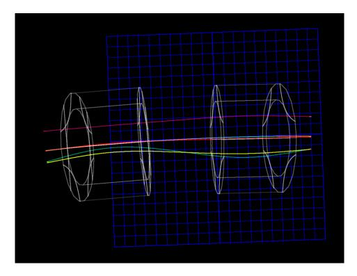
The orbits in QF are arranged in order of increasing energy from inside to outside, so if the tight ~4mm gap between the beam centres and the inside of the vacuum chamber is a problem, it will be the extreme ends of the 20-80MeV energy range that are lost, with intermediate energies still transmitted. Notably the 60MeV orbit stays very close to the circle of the vacuum chamber centre, which is also shown in the figure.
