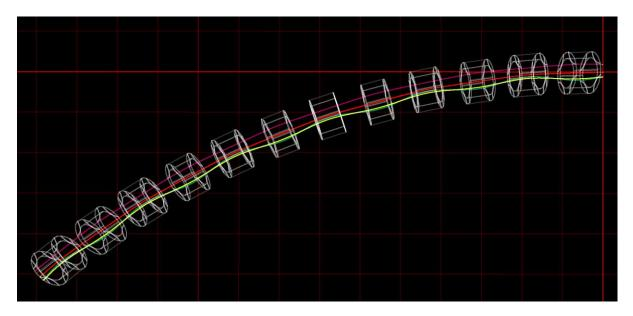
This simulation was done in Muon1 with a soft-edged Maxwellian field model. In studies for the CBETA FFAG arc, good agreement was obtained between orbits using OPERA-3D fieldmaps and orbits using Muon1's model (<1mm difference), although this check will also be redone for this lattice when OPERA-3D fieldmaps for the magnets have been calculated.
