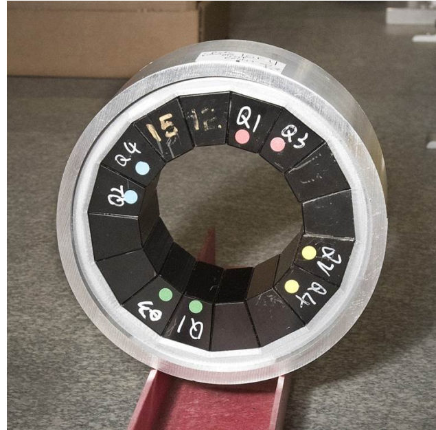
Figure 3: QF magnet without iron wires.
